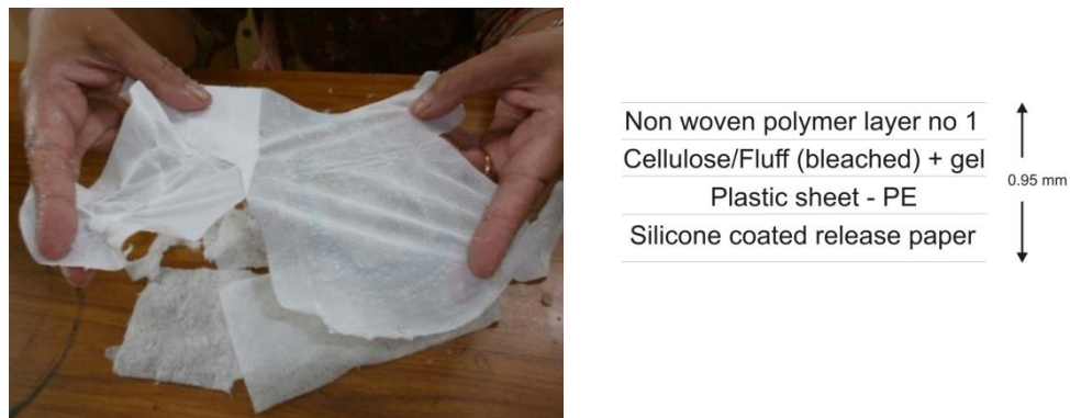
Figure 6 Layers in a pad Source Author Generated
